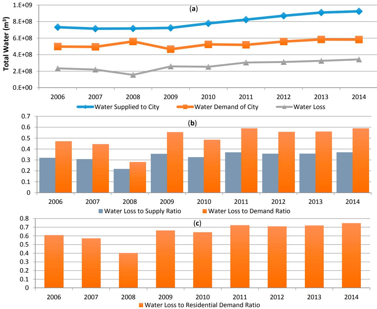
**Figure 2.** Water supply, demand and loss characteristics between 2006 and 2014. (a) Water supply, demand and loss (m<sup>3</sup>); (b) Water loss to supply ratio and water loss to demand ratio; (c) Water loss to residential demand ratio.
